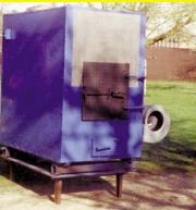
box can reach up to 1,500 degrees, which breaks down the smoke molecules to eliminate smoke. In fact, I can put my nose right over the stack and not smell anything. Gas coming out of the wood gets the proper amount of oxygen which is why the wood burns clean.
