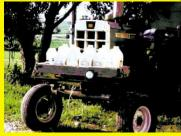
everything from rocks to bags of seed to full or empty pesticide containers. The box is set inside an angle iron frame that's bolted onto the tractor frame. I've used this box for many years. It's really handy. (Dan Knaphus, 66110 150<sup>th</sup> St., McCallsburg, lowa 50154 ph 515 434-2668)
