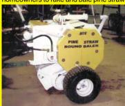
The machines include a self-propelled, hydraulic-driven, 52-in. wide rake, and a 3-pt. mounted, pto-driven round baler. The baler makes bales that measure 15 in. in diameter and 24 in. long. The bales weigh 18 to 24 lbs. so they're easy to handle. An audible signal on the baler tells you when the chamber is full.
