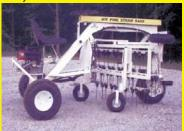
The self-propelled rake is powered by an 8 hp air-cooled gas engine and has a pair of gauge wheels. Cranks are used to regulate ground clearance. A horizontal tree protector wheel on the right side of
