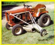
To stabilize my Allis Chalmers 12H riding mower while cutting along road ditches, I made a stabilizer bar from steel pipe and a 10-in. wheel, like the ones used
