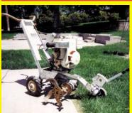
Here's a photo of a sidewalk edger I made from an old tiller. The tiller was ruggedly built and had a good engine.
