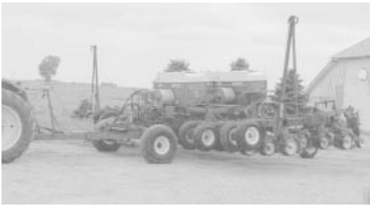
Brian Parkinson combined two IH 12 by 30-in. vertical fold planters. He uses his Deere 8440 4-WD tractor to pull the rig.
