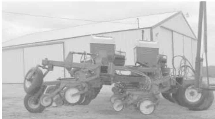
Two seed boxes mount on rear planter bar, and one is center-mounted on the front bar.
