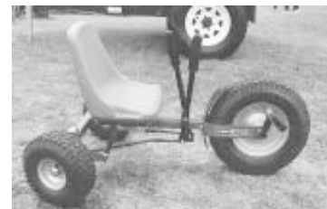
Two joystick levers are used to turn the rear wheels.
