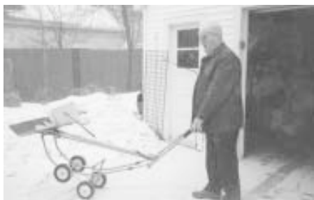
To dump snow off shovel, operator simply reaches down and releases retainer over end of shovel handle. It then pivots up to dump.
