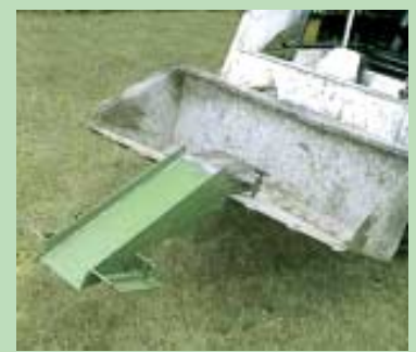
Trenching tool mounts on bucket of skid steer or front-end loader and has skids on the side that allow Rose to precisely control trench depth.
