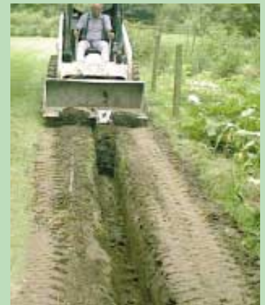
Tool cuts a trench 12 in. wide with no moving parts. It weighs only about 110 lbs. and requires no separate power unit - just a loader.
