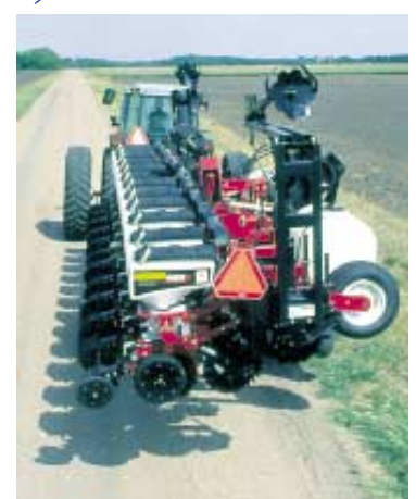
AGCO’s “lift and rotate” cart greatly reduces road transport width.
