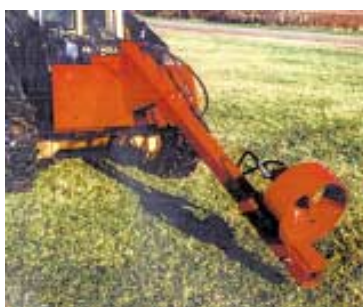
Skid loader-mounted quick-tach boom can be equipped with either a pump or an agitator. Boom is 10 ft. long.
