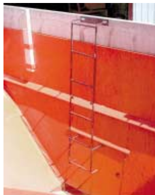
This ladder, made from rerod, hangs over unloading door on a gravity wagon, making it safer to shovel grain out.
