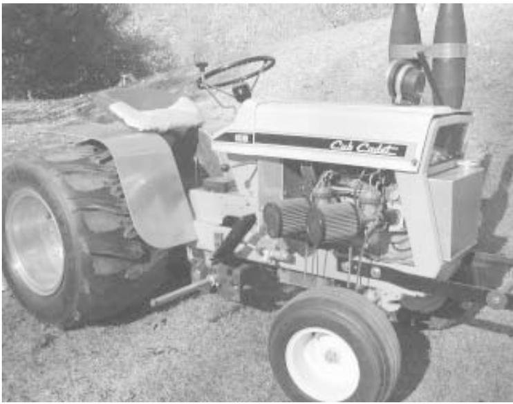
Hasbrouck's 126 Cub Cadet garden tractor is equipped with 31-in. rear "pulling tires".
