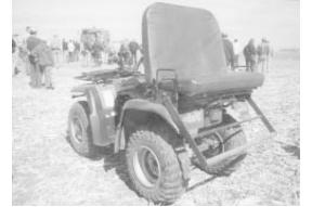
Yamaha ATV is fitted with a school bus seat on back that faces back-ward. Note handles at each side of seat, and foot rests for riders.
