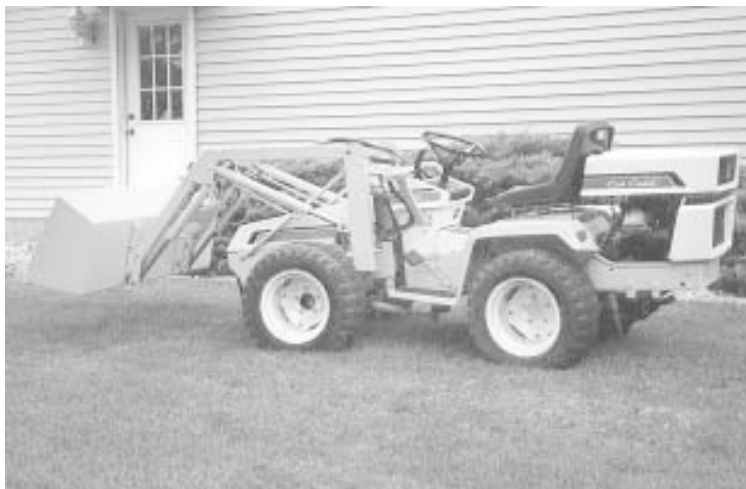
Birkey used parts from Cub Cadet 1250 and 1650 tractors to build this 4-WD articulated loader tractor. It's powered by a 16 hp twin cylinder gas engine mounted on back.
