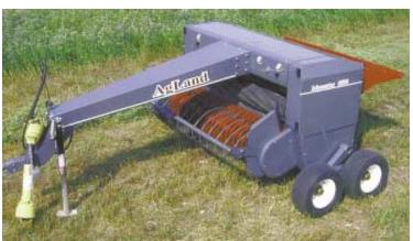
The Macerator 6600 gently nicks stems and leaves, allowing much faster drydown while preserving valuable nutrients and color. Machine has a 66-in. wide pickup.
