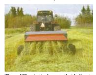
Three diffrent attachments that bolt onto back of machine are available. The one shown above makes the swath come straight down the back of the machine.
