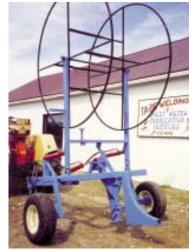
Two-wheeled machine is equipped with a specially designed boot on back that's just 2 1/2 in. wide.
