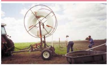
Machine is equipped with a pair of 7 1/2-ft. dia. pipe reels and is designed to lay 1 1/4-in. dia. poly pipe 6 to 18 in. under the ground.
