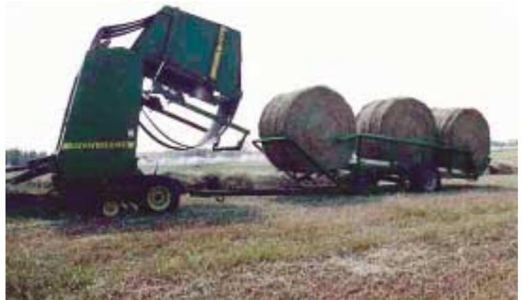
Tow-behind bale accumulator hitches to baler and lets you group bales in threes. It automatically unloads bales out the back.
