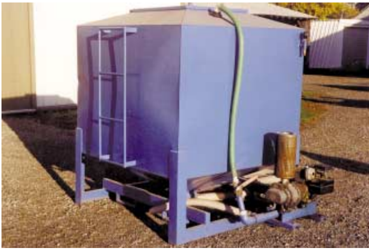
Tank measures 5 by 5 by 4 ft. and holds two mini-bulk bags or pro-boxes. A 3-in. dia. vacuum hose is used to move seed.
