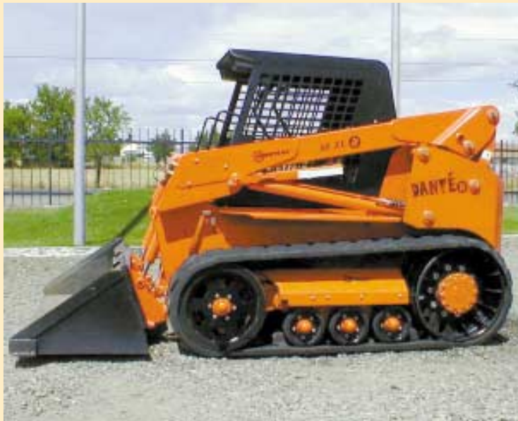
Rubber-tracked skid loader is equipped with 16-in. wide positive drive tracks. Unit is built on a Daewoo chassis minus the power train.
