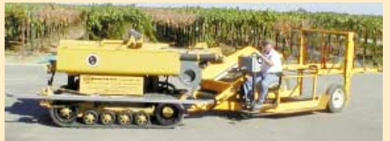
Leading machine is equipped with a platform and can be controlled by “tethers” that run to rear unit.
