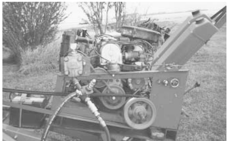
A pulley mounted on transmission is used to belt-drive the auger.
