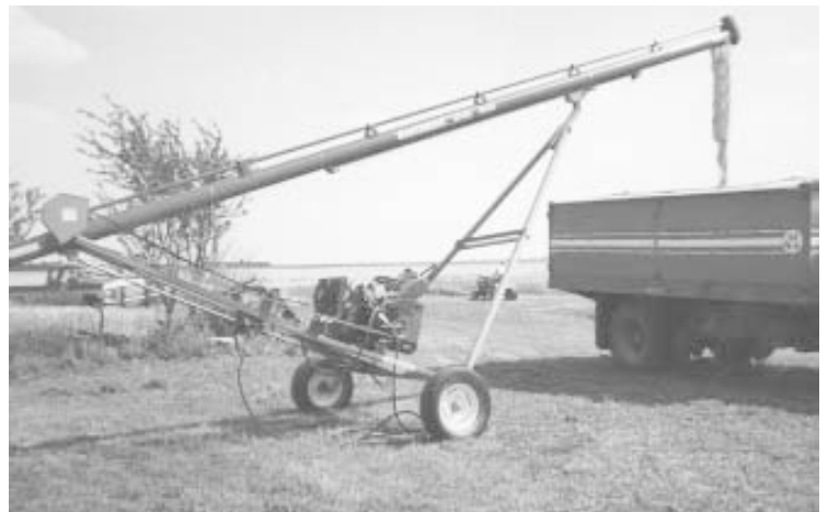
John Gray used a 60 hp gas engine and 4-speed car transmission to boost power and improve performance of his 7-in. dia., 47-ft. auger.
