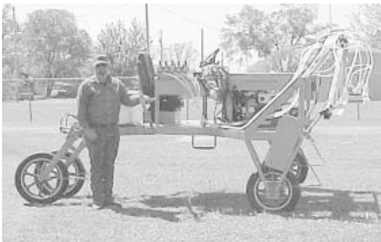
Self-propelled weed wiper is equipped with four narrow motorcycle wheels.
