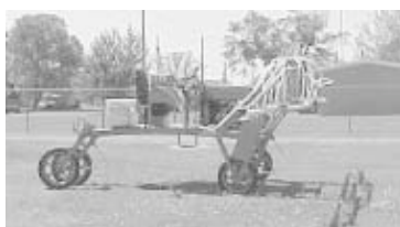
The 2-WD, hydrostatic-drive weed wiper has three front-mount booms that can be hydraulically raised or lowered.
