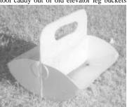
bolted together back to back. The buckets were bolted to each side of a piece of 3/8-in. plywood with a hole cut in the top for a carrying handle."
