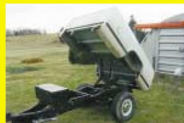
capacity ball hitch, and a trailer connector. A 12-volt powered hydraulic pump mounts in a metal box on front of the trailer to protect it from the weather. There's also a swivel pipe jack on the hitch.
