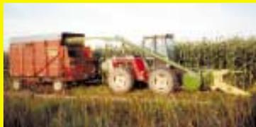
pull-type that we modified to be mounted on and powered by a bi-directional tractor. The harvester can be mounted or dismantled in a few minutes, basically from the tractor seat, so you can use it for other work.
