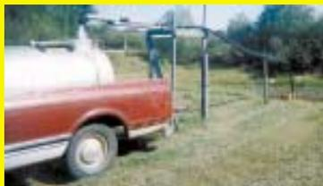
the spout and fill the tank. I just ran the hose over wood supports and put a metal pipe on the end of the hose to act as a nozzle. Saves a lot of time. (Pete Peters, Osler, Sask.)
