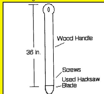
end. A hacksaw blade is bent over the end of the handle, with a gap between the curve of the blade and the end of the handle. The blade is screwed to the sides of the handle and taped in place.
