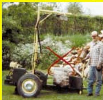
the end of the cable lift the chunk onto the splitting table and hold the chunk in place while you split it.
