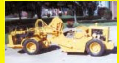
gines are Vanguard series Briggs and Strattons. It's fitted with Sundstrand transaxles taken from older Wheelhorse tractors. The tires are 6-ply.
