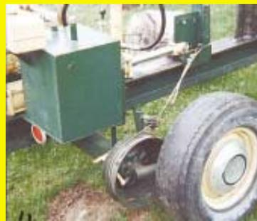
can be adjusted from ground level up to waist height using a cable that wraps about the axle. The cable attaches to a pin on the splitting wedge. When you get the table to the desired height, you just pin the support arms into place.
