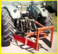
to spend the money for a commercial potato hiller so I built my own, mostly out of scrap metal. It's equipped with a pair of 6-ft. long, 1-ft. high, 3/8-in. thick steel plates that angle back toward a 16-in. wide opening. The back part of the blades is supported by a frame made out of 2-in. sq. tubing. The front part of the blades, which fits just inside the tractor's rear wheels, can be raised or lowered by adjusting a pair of threaded rods.
