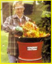
Our new Leaf Eater chopper turns 8 bags of leaves and cuttings into a single bag of mulch. The electric chopper runs on 110-volt power.
