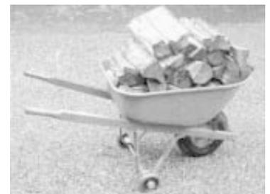
**With three wheels there's less chance of tipping so you can move bulky, unbalanced loads safely and easily, says the company.**
