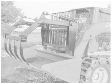
Grapple fork looks like an eagle's claw and can be used for many jobs. It can be quickly removed, allowing you to use the bucket for other work, says inventor Mark Underwood, noting that the grapple teeth are unique because they pivot from side to side.
