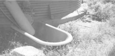
Cast iron tub eliminates need to dig a hole and also keeps grain from spilling onto the ground.
