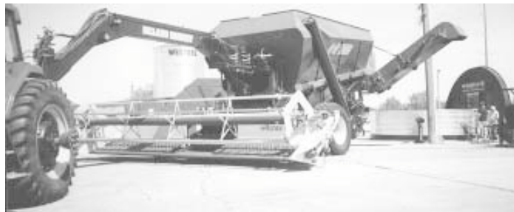
Harvester is essentially a 20-ft. header mounted on a grain tank. Grain is harvested "dirty" in the field and taken back to the bins for cleaning.
