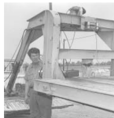
Telescoping hitch allows bed to be tilted for easy loading of machinery.
