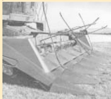
side to adjust to varying conditions. The arms bolt in place which allows the unit to be quickly removed. Arms and bearings have set screw adjustment on a square center tube which stops slippage.
