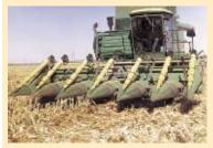
cones lift the crop up and into the cross auger. The company says the simple and lightweight units won't interfere with normal operation. They sell for about \$400 per row.
