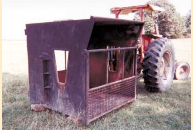
Bottom 2 ft. of gate is covered with 2-in. sq. mesh panel, with three headgates above it.
