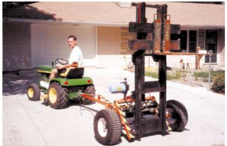
Parker built this two-wheeled "tow behind" forklift out of a commercial forklift mast.
