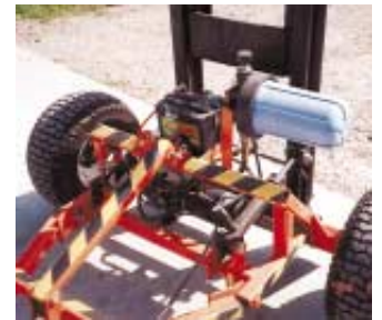
Parker built this two-wheeled "tow behind" forklift out of a commercial forklift mast.
