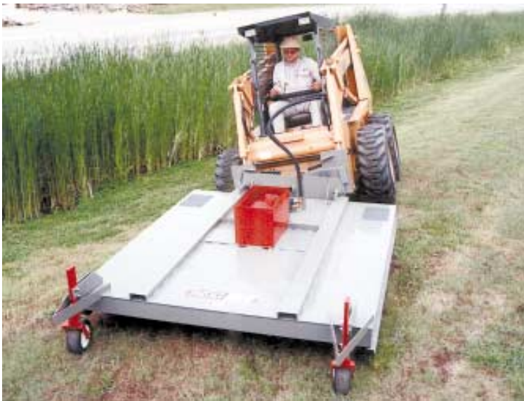
Hydraulically-powered mower has a cutting width of 61 in. Deck pivots from side to side and up or down.
