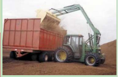
Loader has a 17-ft. lift height for loading into high-sized trucks.
