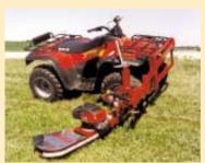
Spring and torsion guide system automatically adjusts deck to ground contour.
