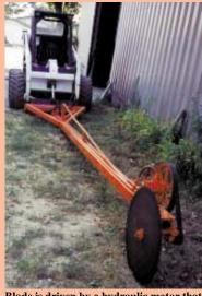
Blade is driven by a hydraulic motor that operates off loader's hydraulics.
