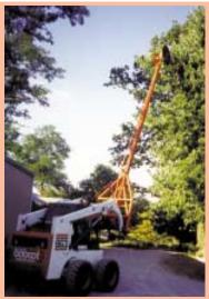
Skid loader-mounted saw can reach up to 25 ft. to trim overhanging branches.
