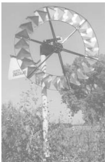
**Delta Jr. windmill is equipped with an 8-ft. rotor with 24 galvanized steel blades.**
