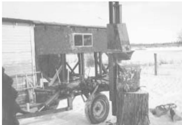
**To split wood, Kuefler simply bolts a homemade splitting wedge to base of post pounder's hammer.**
