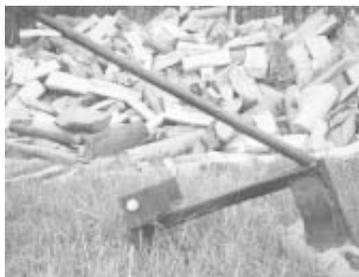
**Homemade wedge - an old axe head - welds onto an angle iron bracket that fastens to bottom of post pounder's hammer.**
