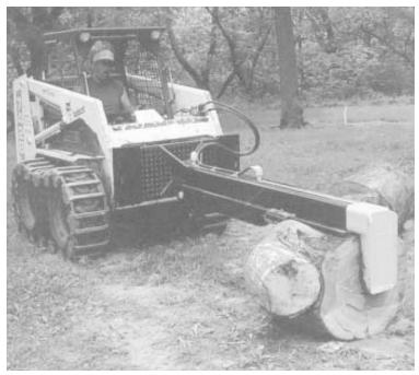
"It can pick up, move, and split heavy logs without the operator ever having to touch the log," says Lawrie about his skid loader-mounted splitter.
