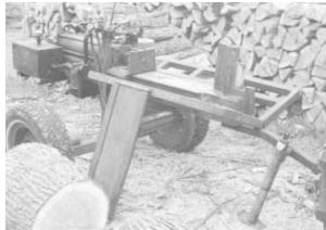
Two-wheeled machine is equipped with a self-loading lift arm on one side that lowers all the way to the ground and lifts big chunks of wood onto splitting table.
