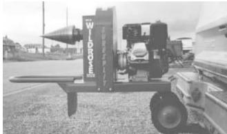
Pto-powered rotary splitter mounts on wheels so it can be moved around easily.
