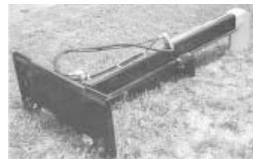
Unit is equipped with a quick-tach universal mounting plate. It operates off loader hydraulics.
