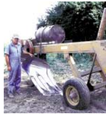
Lay built his deep ripping "spader" by fastening 4-ft. long sections of road grader blade lengthwise to bottom of shanks.
