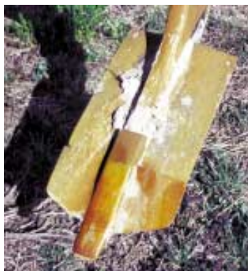
On the three shanks he lengthened, Bauer welded sections of 10-in. wide hardened steel grader blade.
