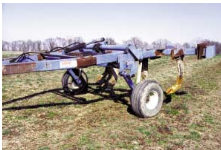
Bauer converted a prototype DMI Turbo Tiger into a five-shank "spader".
