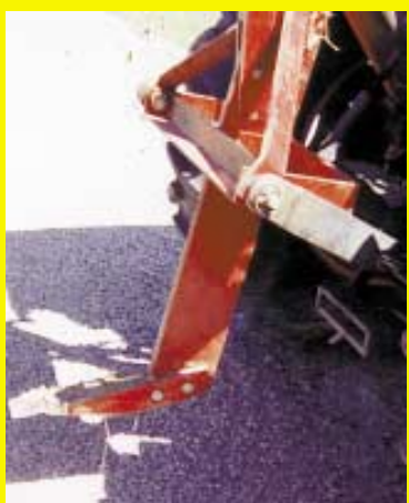
Tractor-mounted rock digger consists of a subsoiler shank mounted backward on a frame that fits a 3-pt. hitch.
