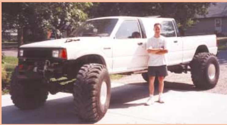
Jeff Parker built his own extended cab pickup by welding together two Mazda 2-WD half-ton pickups. The machine is 21 ft. long with a 6-ft. bed and rides on 44-in. tires.
