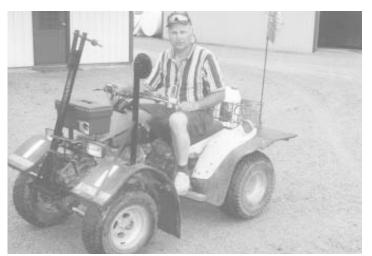
Robert Dunton got tired of mud flying up at him while checking irrigation equipment. He solved the problem by making fenders out of used rubber conveyor belting.
