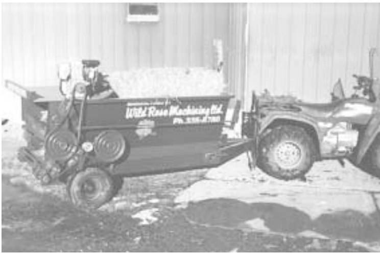
Miniature spreader measures just 3 by 6 ft. and 24 in. deep. Scott pulls the spreader with either a garden tractor or ATV.
