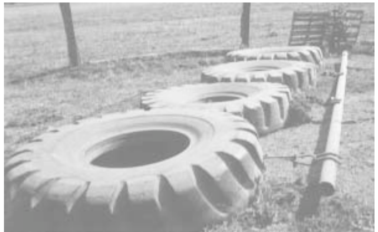
Hurlimann's 24-ft. wide drag is made of two 29-in. wide used loader tires, each about 6 ft. high. He sliced the tires in half with a chain saw.
