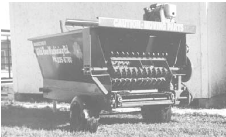
Aggressive chopper/beater bar has steel flails set at angles in a rotating drum.
