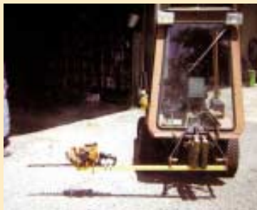
Chain saw extends about 5 ft. to side of tractor, allowing Baldwin to cut weeds along a railroad right-of-way.
