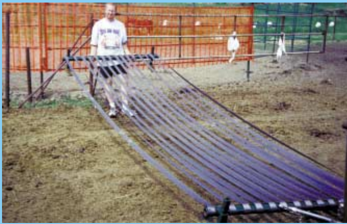
No-pit guard is made from a series of 2-in. wide polyester belts attached to two steel pipes. A crank on one end of pipes is used to stretch belts and raise them off ground.
