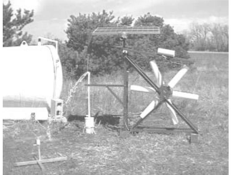
Solar-powered pump has a walking beam/rocker arm design similar to that of oil well pumps. Concrete-filled flywheel kicks in at 40 rpm's to boost efficiency.
