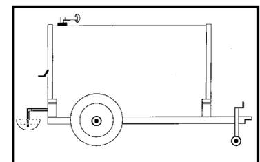
As animals drink they lower the water level in trough, which causes discharge pipe on back of tank to suck air into tank, releasing more water down the pipe.
