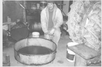
"It's easy to move around and will hold more than 30 gallons of oil," say Roger and Bruce Elliott about the 3-ft. dia, oil drain pan on wheels they built.
