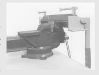
field on a pickup-mounted vise to make brackets from strap iron or bend sheet metal into repair or replacement panels, covers, etc.
