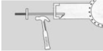
chisel tip onto the inside. Then pound on the sq. tubing with a hammer to pull it out."
