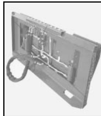
**"Quick Change 2000" mounts on any skid loader equipped with universal quick tach mounting brackets and is equipped with a pair of spring-loaded pins operated by hydraulic cylinders. It eliminates the need to get out of the cab and manually latch or unlatch pins.**
