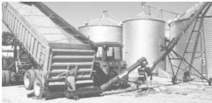
**Tractor pto-drives auger at a right angle, which leaves room for a semi trailer to pull right in alongside tractor. Jacobs then pulls swing-away unit into place behind truck.**
