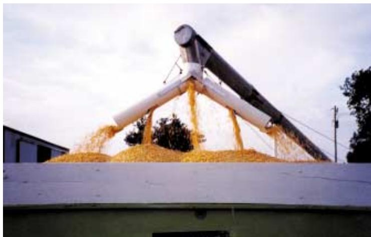
Five streams of grain flow from the “Grain Levelor”, which attaches to auger spout.
