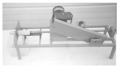
Electric-powered sweet corn stripper is equipped with a plunger that pushes ear through a dye that has a sharp edge all the way around it to shear kernels off.
