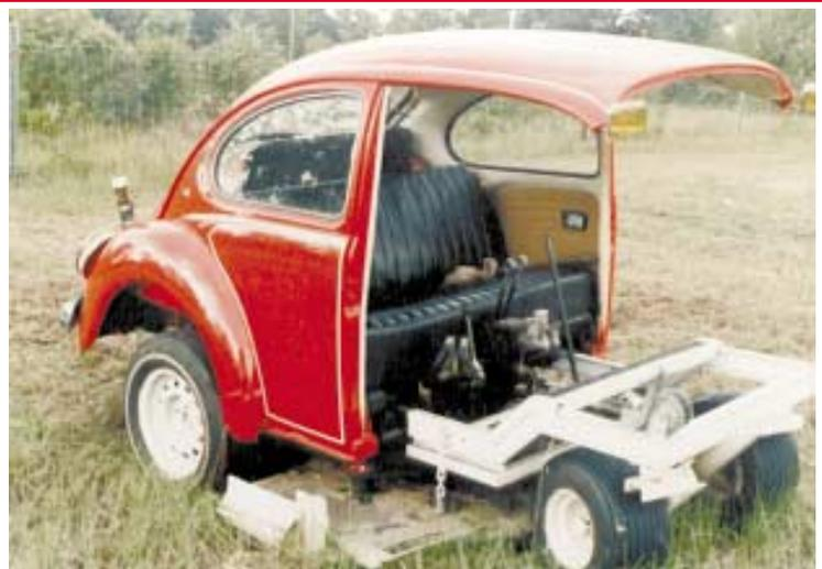
**Howard Blakely used the back end of a 1973 VW Beetle, which let the operator ride in comfort.**
