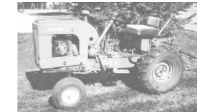
**Deere “L” look-alike is powered by a 20 hp, 2-cyl. engine off an old pull-type combine.**
