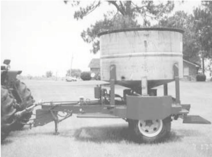
Randy Thompson's machine is equipped with a stainless steel, hopper-bottom fertilizer mixer tank. Infrared sensors help fertilize two rows of trees at once.
