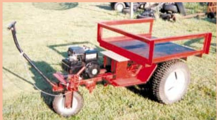
Made from an old Wheelhorse riding mower, Chumley's wheelbarrow is powered by a 5 hp gas engine.
