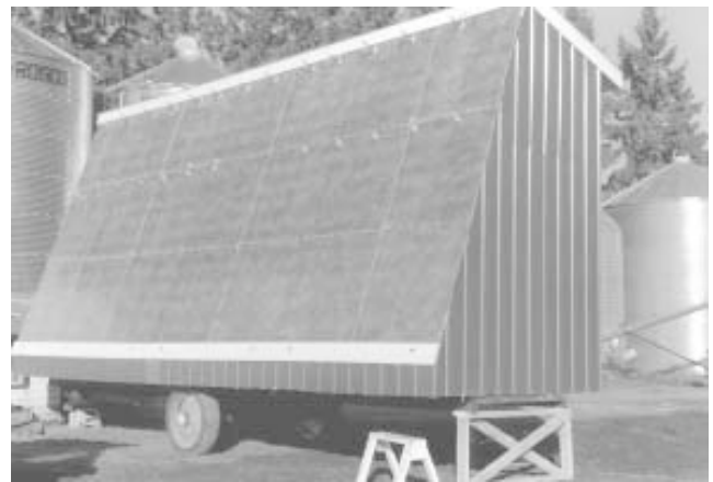
Solar grain dryer measures 12 by 28 ft. and has a transparent fiberglass face inclined at a 70 degree angle.
