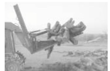
Optional "tweezer grapple" allows operator to grab and hold several trees on snout of saw.
