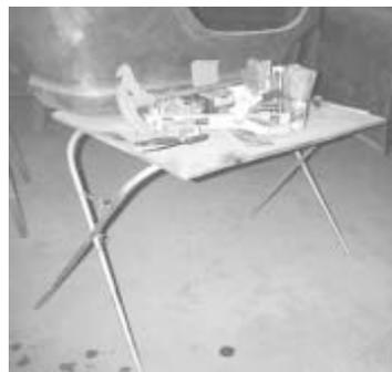
To make benches, Douglas simply bends conduit at right angles to make legs.
