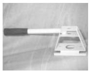
You put your socket wrench through the center to reach the bolt and hang onto tool's rubber-gripped handle.
