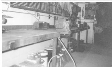
Gilbertson welded two 20-ft. sections of steel I-beams together to make this 20-ft. long, 30-in. wide workbench. Note receiver hitch built into bench (at left in photo).
