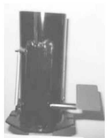
Flow monitor consists of a 6-in. dia. steel tube equipped with a mechanical flow valve that has a bright orange flag attached to it.
