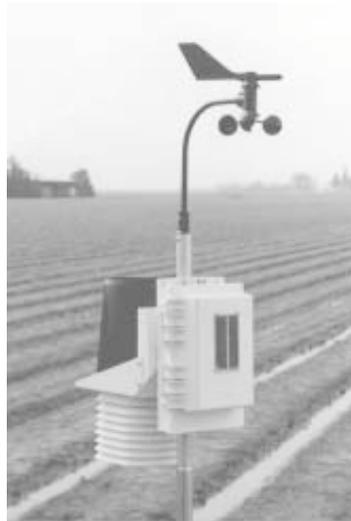
Wireless weather station is powered by a built-in solar panel. It transmits data to remote display console.
