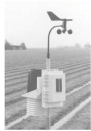
Wireless weather station is powered by a built-in solar panel. It transmits data to remote display console.
