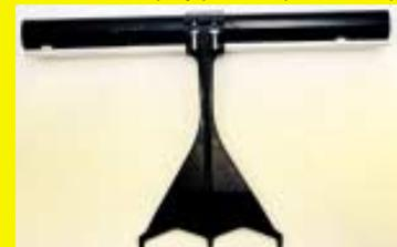
into the header and keep the cutter bar cleaned off, which results in even feeding of the crop into the combine. They work great on soybeans, cereal crops, and short specialty crops. The paddles
