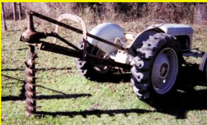
Years ago my dad and cousin cut part of the rear end off a pickup and attached it to a 7-in. dia. post hole auger that's pto-driven off our Ferguson 20 tractor. They cut off part of the axle on each side of the differential, then drilled a hole through the stub shaft and bolted the auger shaft on. They made their own pto shaft and attached it to the differential's yoke. A
